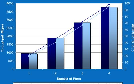
**Test** Netperf 2 Clients Per Port Under Test TCP STREAM TEST Buffer Sizes = 64K Bytes 60 second test iteration 64KB Socket Size **Data Verification Enabled** \*(Touched Data) **Bensley Server** Intel® Bridgeport CRB 55 2x 3.2GHz Dual-Core Intel® Xeon® processor 8GB RAM Linux Kernel 2.6.16.1 patched with Intel® I/OAT DMA v1.5 Base Driver 7.0.38 Clients Dell PowerEdge 1750 3.4GHz Pentium® 4 processor Windows XP Professional SP1 **Network Configuration** Cisco 6509 Clients connected @ 1000 Mbs
